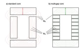
Fig. 1 Run of flux in: a) standard core, b) multi-gap core  $\Phi_G$ -main flux,  $\Phi_R$ -leakage flux
